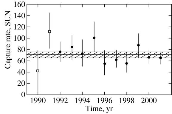
**Fig. 5.** Results of the measurements combined by years; open and filled symbols refer to  $K$  and  $K + L$  peaks, respectively; the hatched region corresponds to the SAGE result of  $70.8_{-5.2}^{+5.3}$  SNU. The data shown have a statistical error of 68%.
