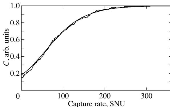
**Fig. 4.** Cumulative distribution functions for the neutrino capture rate measured in 158 SAGE data sets (histogram) and calculated by the Monte Carlo method (solid line). The capture rate in Monte Carlo calculations was taken to be 70.8 SNU.
